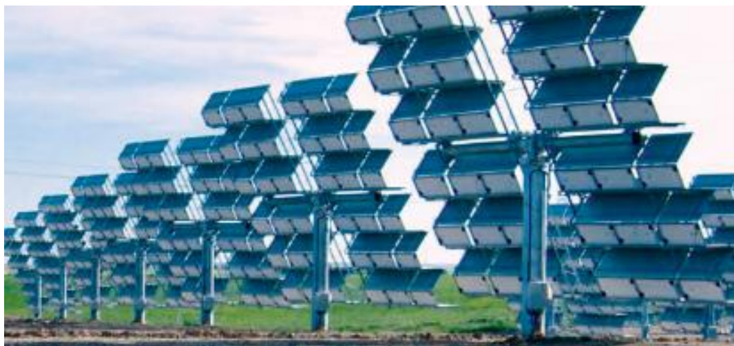
Solar tracking: 2 axis ( and concentration)
